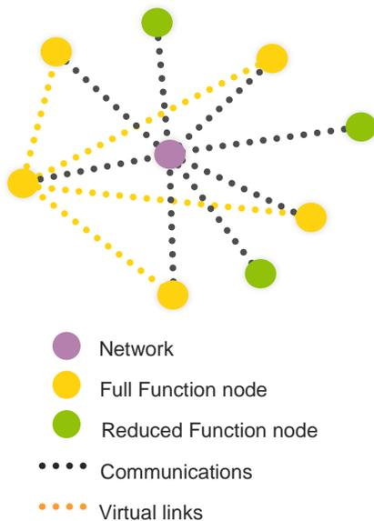
Fig. 10. ZigBee Mesh Networking
