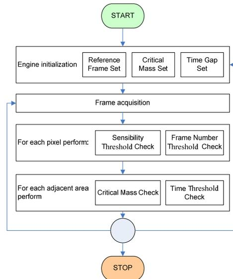
Fig. 5 SICIS Detection engine steps
